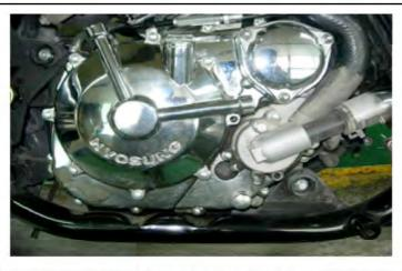
FRONT EX PIPE is disassembled.
