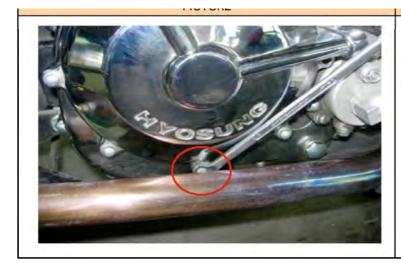
If you operate this replacement without AIR TOOL, you do not need to disassemble FRONT EX PIPE.(Refer to PIC)
