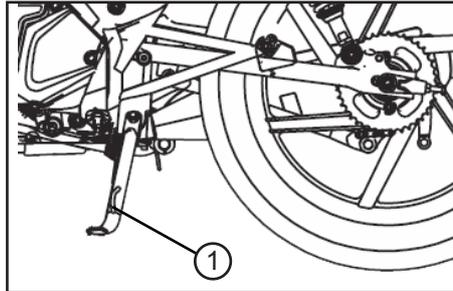
The side stand (1) is located on the left side of the vehicle. Release the side-stand by using your feet to step on the
