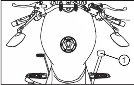
The brake pedal (1) is located on the right-hand side of the vehicle and operates the rear brake. Familiarise yourself with how it works before you ride the vehicle on public roads. Novices and returning riders are recommended to take a riding techniques course.
