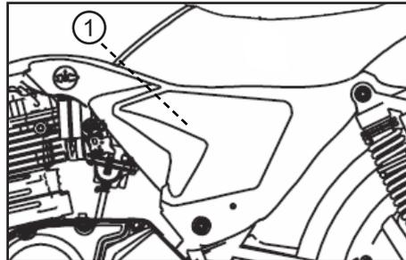
The air filter (1) should be replaced according to the maintenance schedule.
