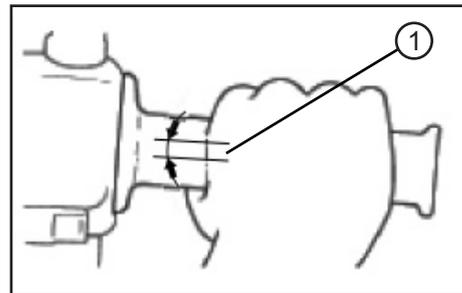
The throttle cable free play (1) should measure 1.5 ~ 3.5 mm at the throttle grip.
