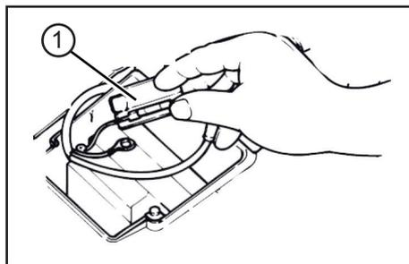
The fuse holder (1) is located behind battery.
