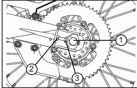
**Tightening torque of the collar nut (1): 70 Nm**
