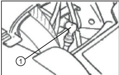
3. Remove the spark plug as shown, with the spark plug wrench (2) included in the owner's tool kit.
